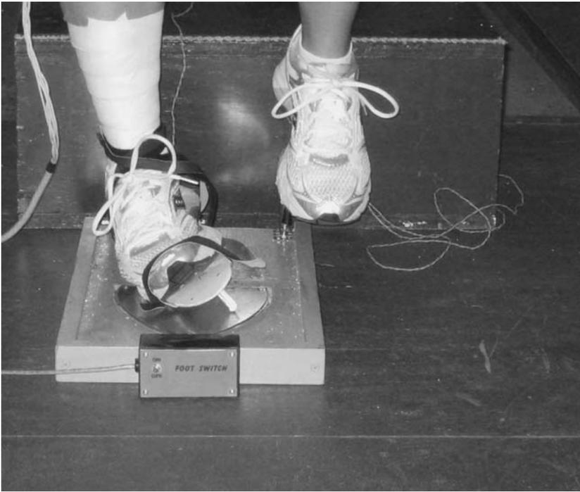
Figure 2. Contact of lateral border of outer sole with metal landing area, indicating completion of the 25° of inversion.
