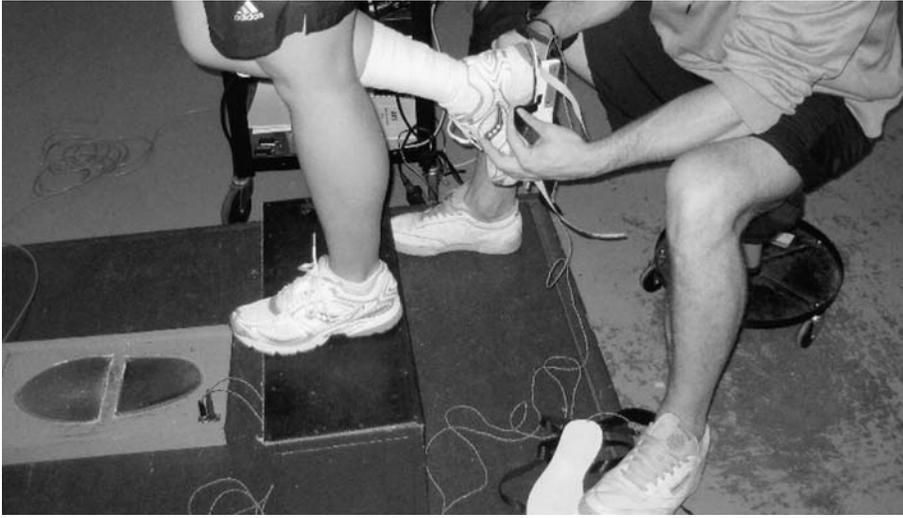
Figure 4. Placement of testing foot behind the participant to strap on the outer sole.
